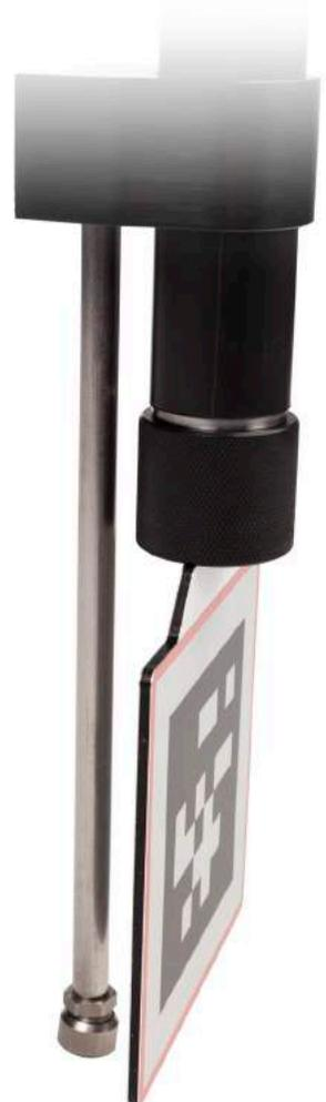
*Above:* A special "foot" on the vertical scale bar keeps the April tag off the ground, allowing the bar to lean against any vertical surface.
